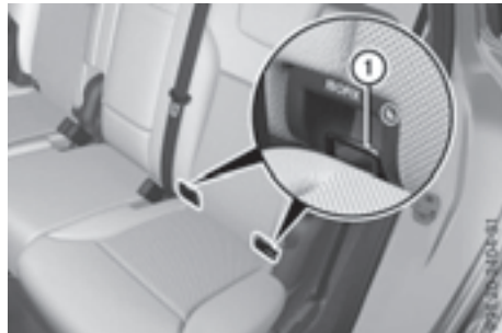
LATCH-type (ISOFIX) securing rings for the outer seat in the second row of seats
