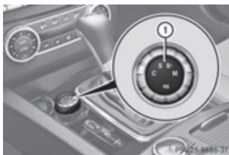
Drive program selector with manual drive program
